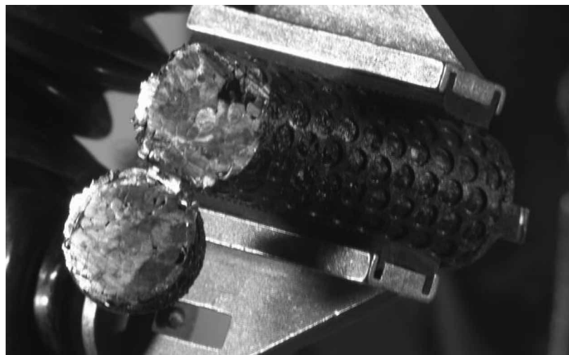
Figure 9. Post-test fuel section of the first electrolytic reduction run with BR3 spent oxide fuel.
